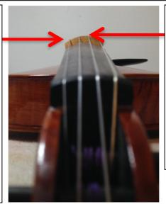
The top of the bridge should be shaped into a nice curve. Too flat will make playing on only one string difficult. The bridge curvature should mirror the curve of the fingerboard, with the string clearance on the E string (the top string) being slightly lower than the G string (lowest string).
